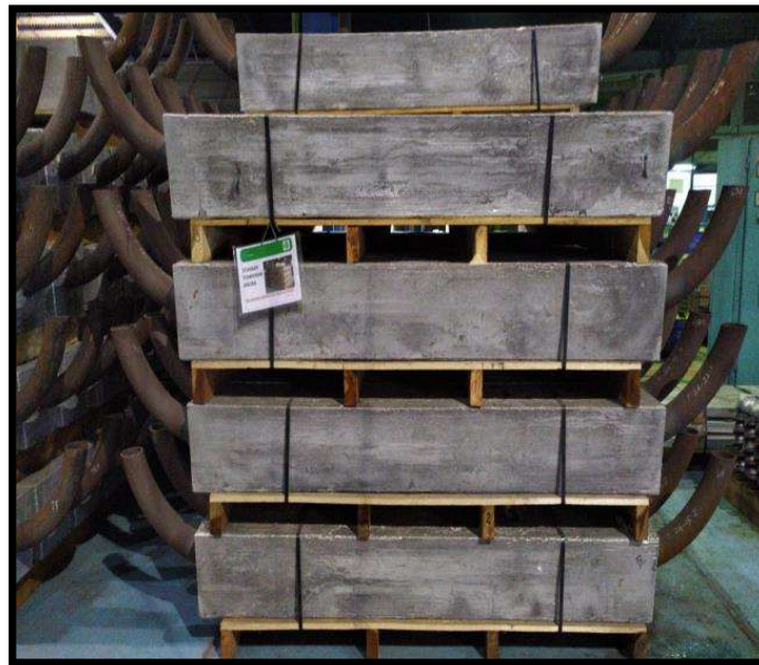
STRUCTURAL JETTY ANODE
